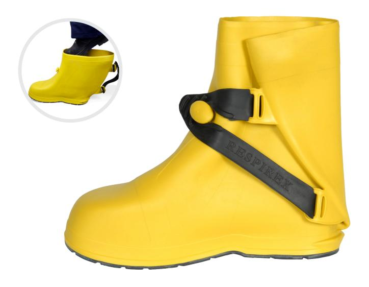
Maxi dielectric overboots incorporate a unique rear opening design that makes it easier for wearers of large or bulky safety boots to fit. With a hard wearing and slip resistant vulcanised rubber sole the maxi overboot provides protection of up to 20kV over the complete boot for over three minutes.
