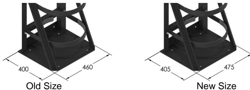
NO CHANGES have been made to any of the mounting hole locations. The improved bracket can be used to replace an old bracket providing there is adequate clearance for the base plate.
