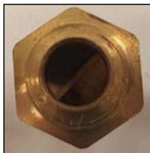
**Figure 2 – Old PEFS BM17 nozzle (rear view)**
