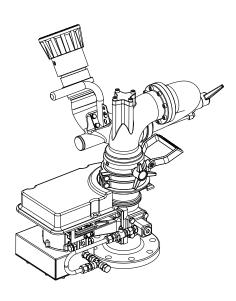
A sealed for life gearbox is provided with adjustable sweep angle between 45° and 120° in 15° intervals and an oscillating speed control. Low friction joints ensure easy movement even at high operating pressures. A highly efficient pelton wheel water motor uses small quantities of fire main water to provide power for automatic oscillation.
