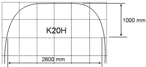
Typical K20H pattern at 4 bar when mounted 250mm away from tank shell.
