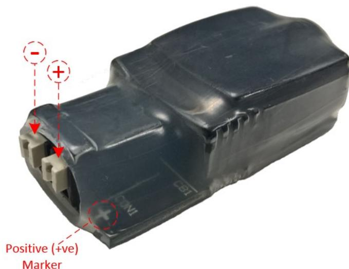
*Figure 2 - Tester Polarity*
