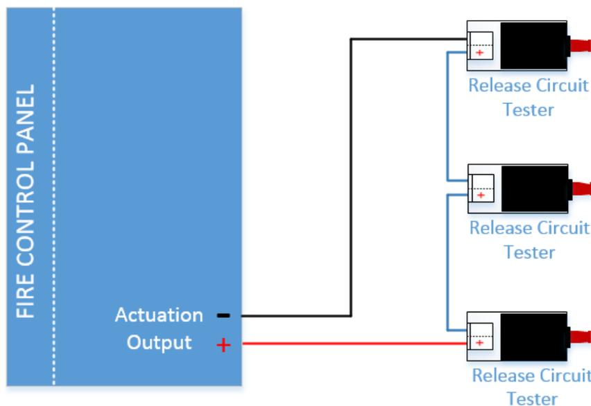
*Figure 3 - Connecting Multiple Testers*
